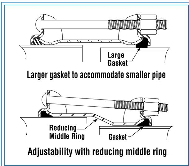
**Dresser Transition Couplings** permits you to connect two different kinds of pipe or sizes of pipe. You simply select the correct coupling for the different pipe diameters being joined. The drawings at left illustrate how gaskets of different cross-sections adjust the coupling to suit your requirements. Further adjustment is accomplished with reducing middle-ring couplings. Please consult factory for size specifications for your particular requirements.
