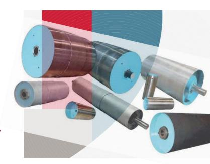
The Magnetic Head Pulley replaces the head pulley of a conveyor and is available as either a Permanent or Electro model. In both designs, the magnetic field covers the entire 360-degree circumference of the pulley, ensuring that conveyed material is fully exposed to the magnetic extraction force at all times.
